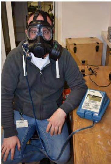
**Figure 18.** Checking the fit of a mask, using a PORTACOUNT (author's photo)
