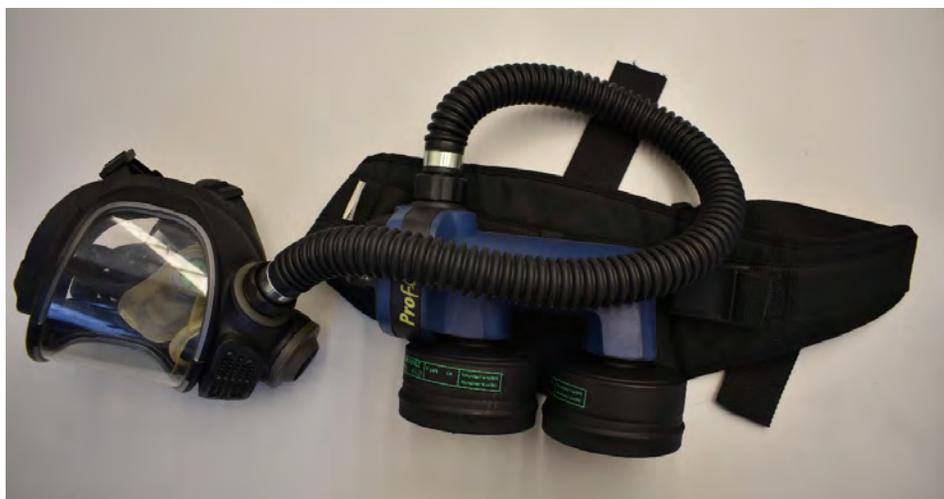
**Figure 17.** Mask with an extra airflow system (author's photo)
