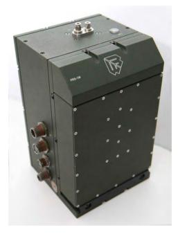
**Figure 19.** PRS 1W – Differential Mobility Spectrometer for CWA and TICs detection, for mounting in vehicles and fixed installations (author's photo)
