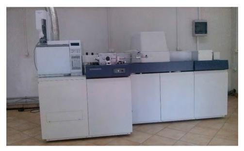
**Figure 29**. Micromass Autospec GC – HRMS (High Resolution Mass Spectrometer) (author's photo)
