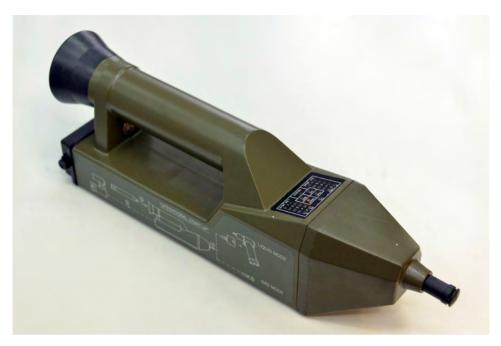
**Figure 16.** A Proengin AP4C FPD field detector, with an S4PE liquid sampler (author's photo)
