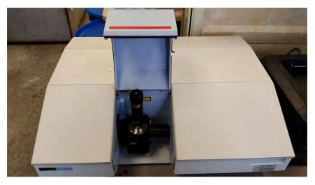
Figure 22. Spectrum BX FTIR Spectrometer (author's photo)
