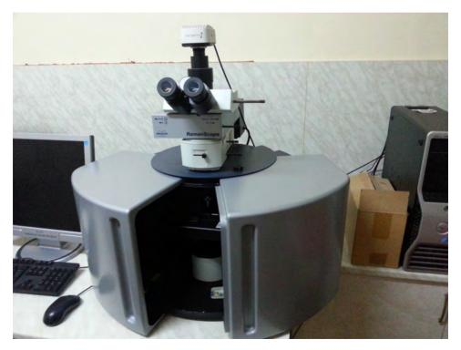
**Figure 27.** Bruker RamanScope III (author's photo)
