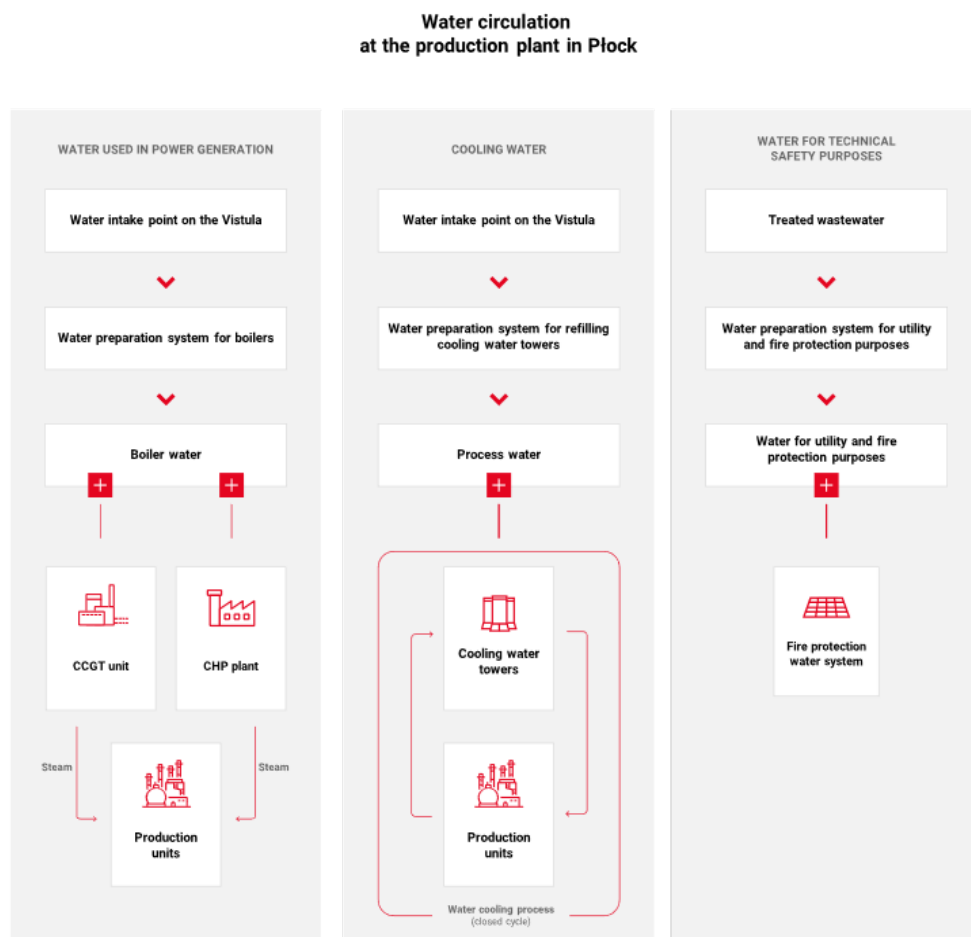
Figure 1. Water circulation in the Płock Production Plant
