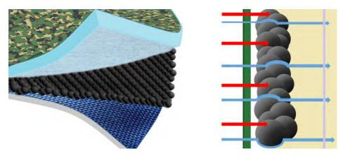
Figure 15. SARATOGA material with spherical, activated carbon
