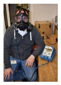
Figure 18. Checking the fit of a mask, using a PORTACOUNT (author's photo)
