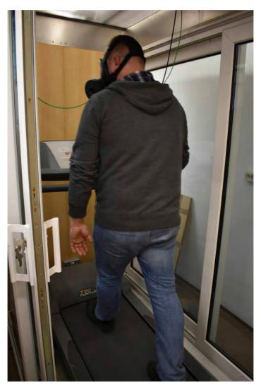
Figure 19. Checking total internal leakage (author's photo)
