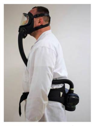
Figure 16. Mask with an extra airflow system (author's photo)
