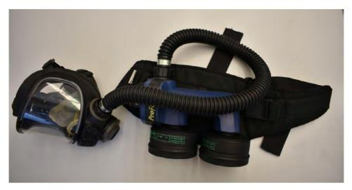
Figure 17. Mask with an extra airflow system (author's photo)
