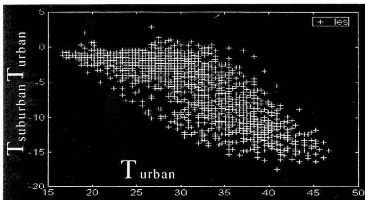
Fig. 2. Hourly temperature differences between the Ippokratous urban station minus the reference station as a function of the temperature of the urban station for the period June to September 1996. Data refer to day and night period
