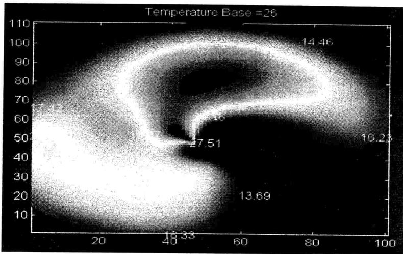
Fig. 9. Spatial variation of the peak cooling load of a reference building in Athens during August 1996 and 26°C set point temperature. Values are in kW
