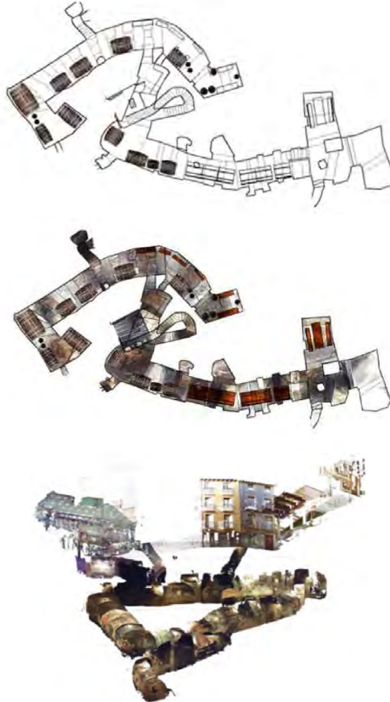
Figure 4a, 4b & 4c. Outlines extracted from the drawing software. Superimposed image. 3D computer graphics in high quality
